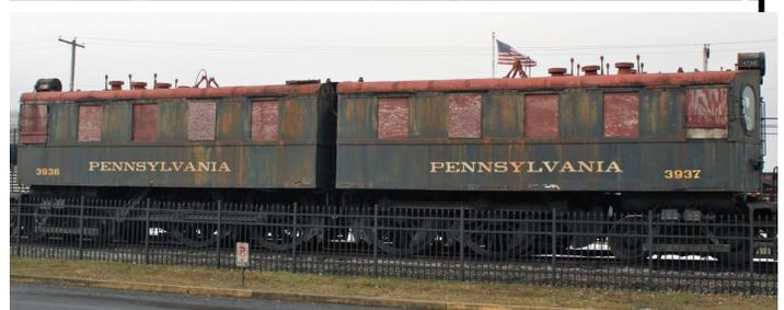
opened in 1910, a new type of locomotive was needed to operate through the Hudson and East River tunnels; a locomotive that wasn't steam powered. Initially the locomotive set used third rail for DC power. Interestingly, they also had an overhead power pole (looking like a very small pantograph) for use when traveling over switches where there was no track level third rail.
