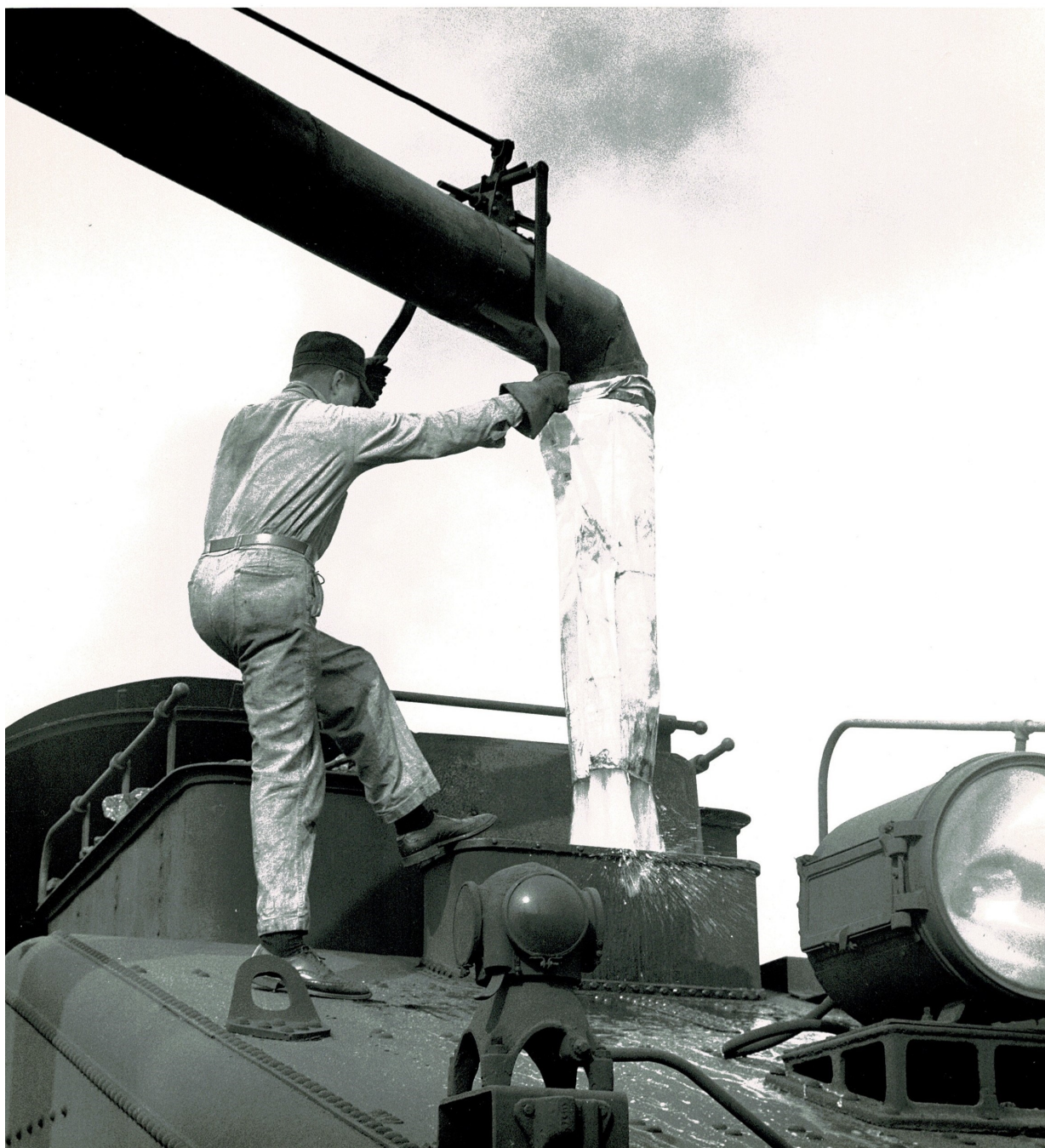
Water replenishment on PRR steam locomotive at Camden NJ on October 1, 1955. Fred Schneider III photo.
