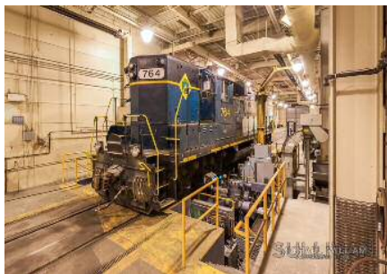
MAINE EASTERN NO. 764 ON THE WHEEL-TRUING MACHINE AT NJ TRANSIT SHOPS BEING READIED FOR SERVICE IN STRASBURG, PA. - MICHAEL WILLIAM SULLIVAN
