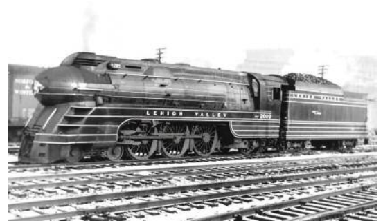
LEHIGH VALLEY No. 2089, A CLASS K-6B PACIFIC-TYPE, STREAMLINED FOR THE BLACK DIAMOND AT SAYRE, PA. ON JANUARY 28, 1940
